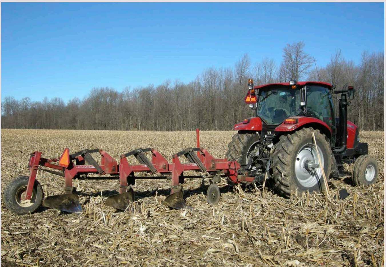
Figure 17. A moldboard plow set to perform primary tillage following a high residue crop. Strip-tillage provides cost savings in such situations.
