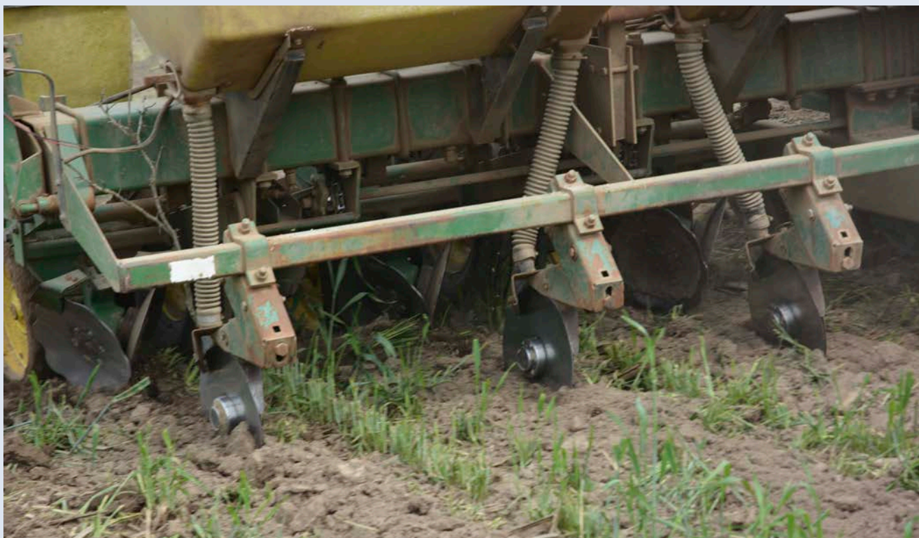
Figure 13. An Ontario planter set up for strip-till conditions. Fertilizer openers help planters stay within the soft strip.
