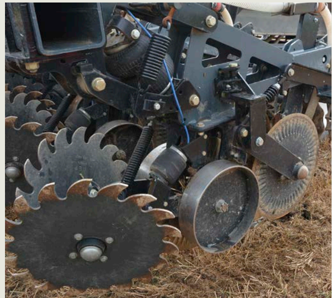
Figure 3. Toothed row cleaner (bottom left) on a strip-till unit.
