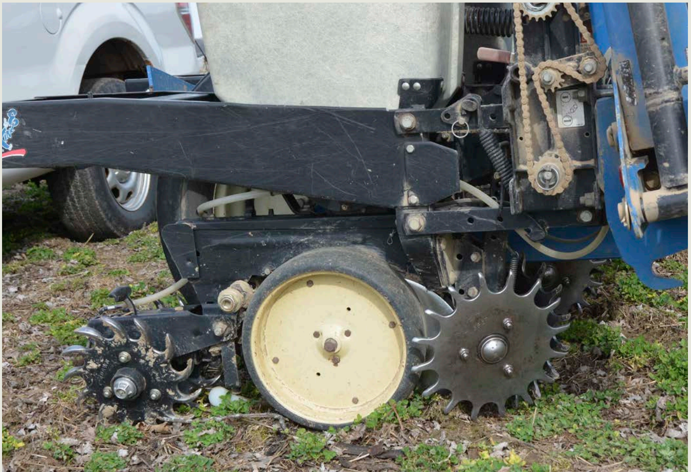
Figure 4. Planter row unit for an Ontario strip-till farmer who plants into one-pass fall strips. Row cleaners on planter remove any residue that accumulates on the strip over winter.
