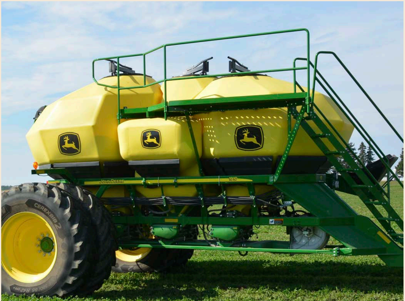
Figure 8. Multi-bin air carts could enable crop-safe, deeper placement of nitrogen and separate placement of other nutrients mixed throughout the strip.
