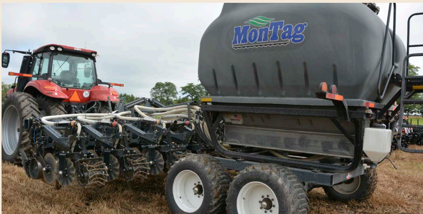
Figure 5. A strip-till unit with an air cart attachment is used to apply fertilizer in strips.
