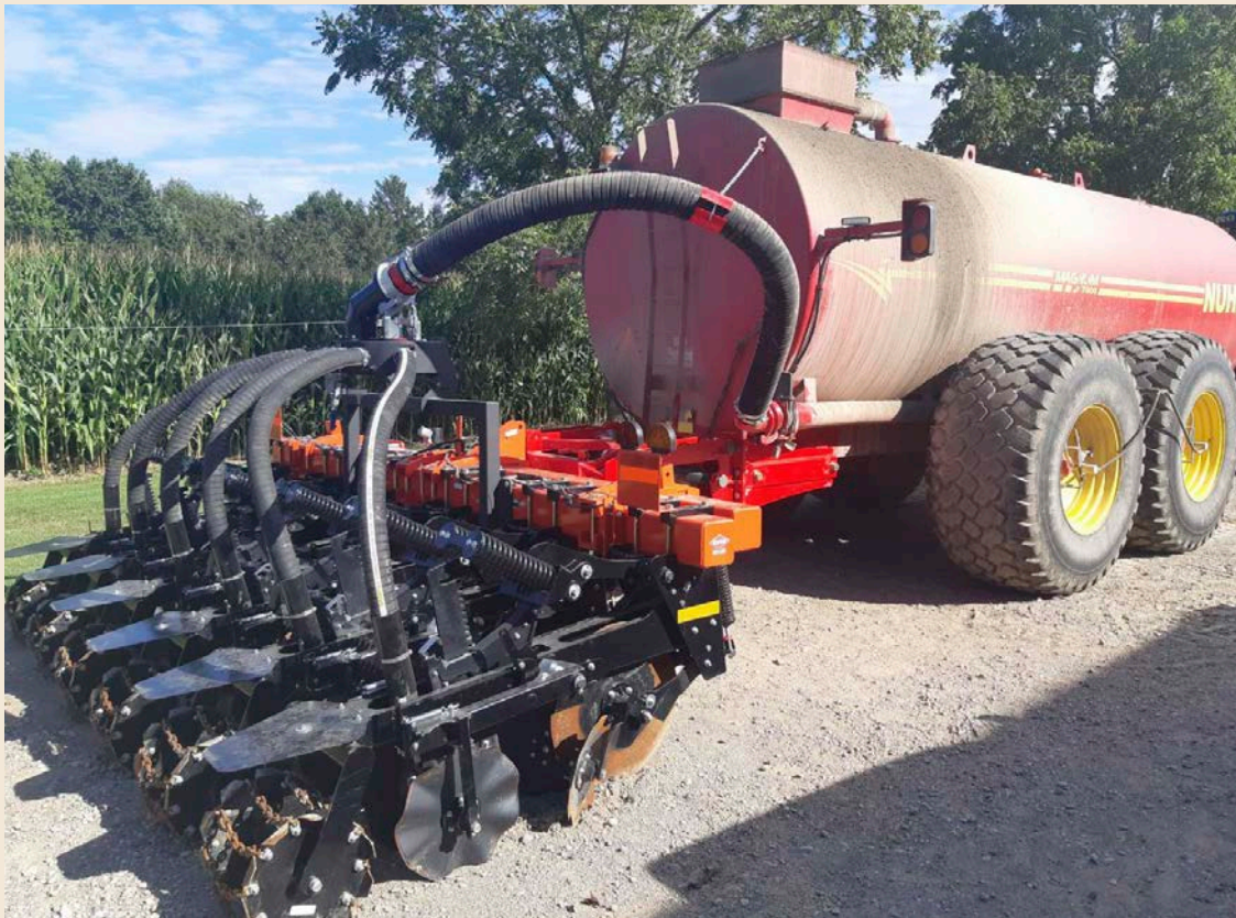
Figure 9. A strip-tiller-manure tanker combination used by an Ontario farmer to incorporate liquid manure.
