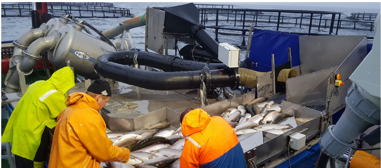
Figure 9. In-water electric stunner. Source: Ace Aquatec, Scotland.
